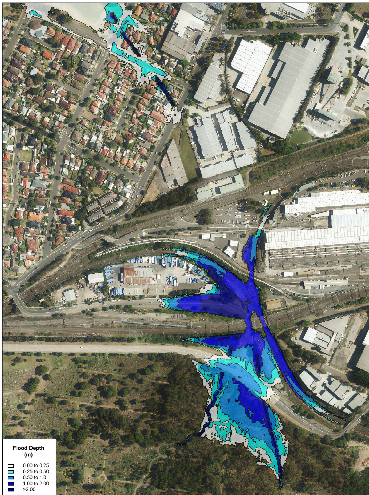
FIGURE C3 Design Scenario - 1% AEP + Climate Change Flood Depths
