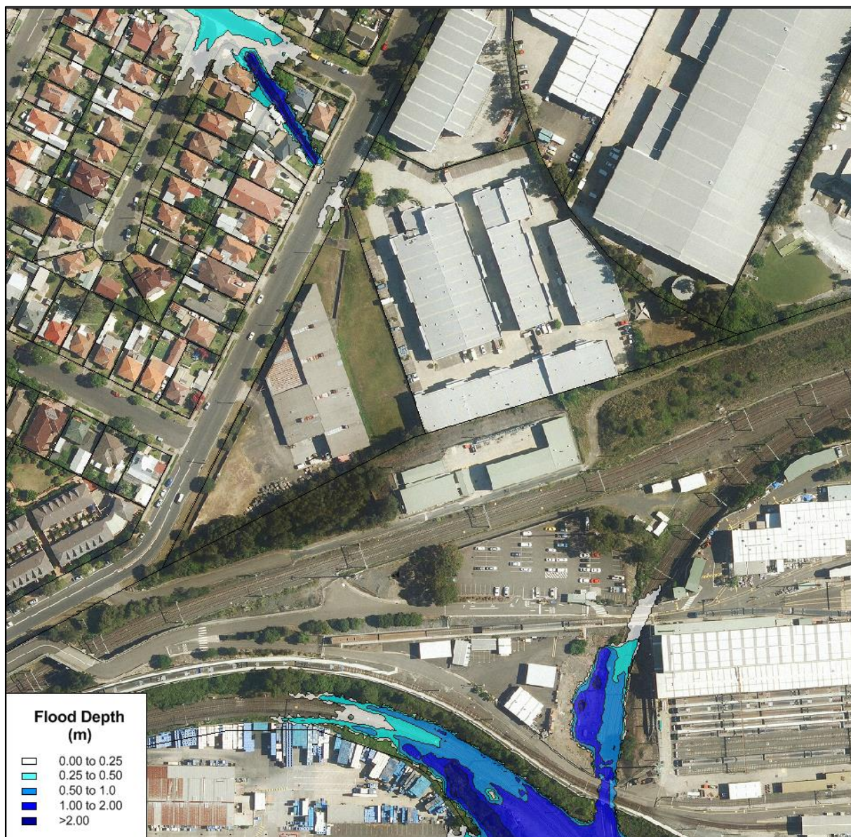
Plate 5-3 – Design conditions flood depth plot 1% AEP event
