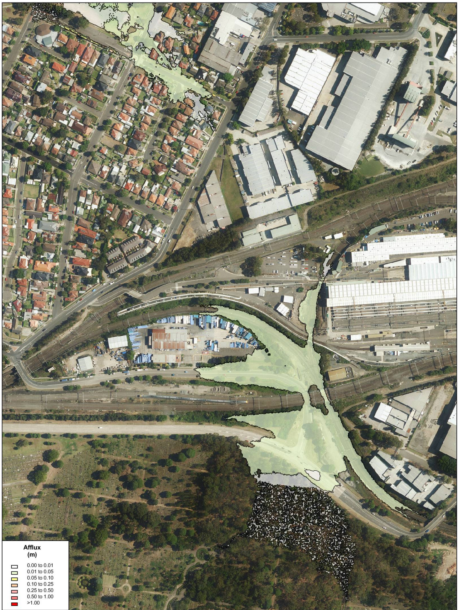
FIGURE D3 Impact Plot - Change in 1% AEP + Climate Change Flood Depths
