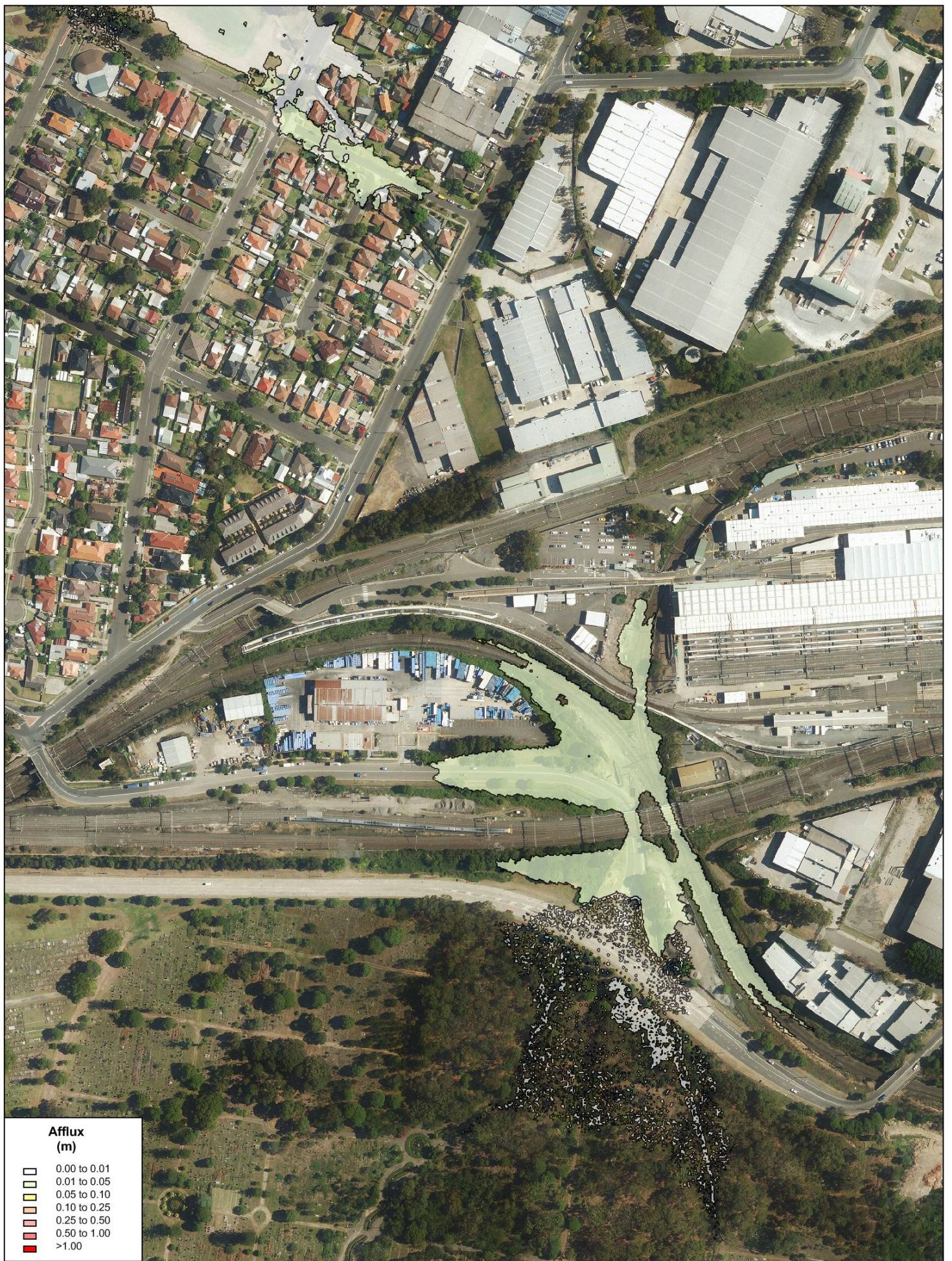
FIGURE D1 Impact Plot - Change in 5% AEP Flood Depths
