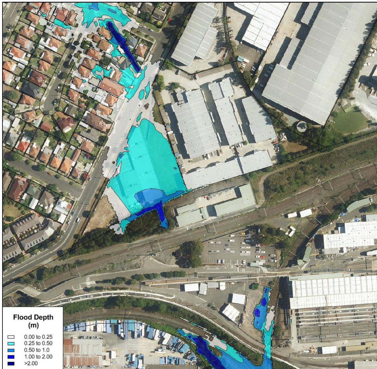
Plate 5-5 – Design conditions flood depth plot 1% AEP event – TestCase1
