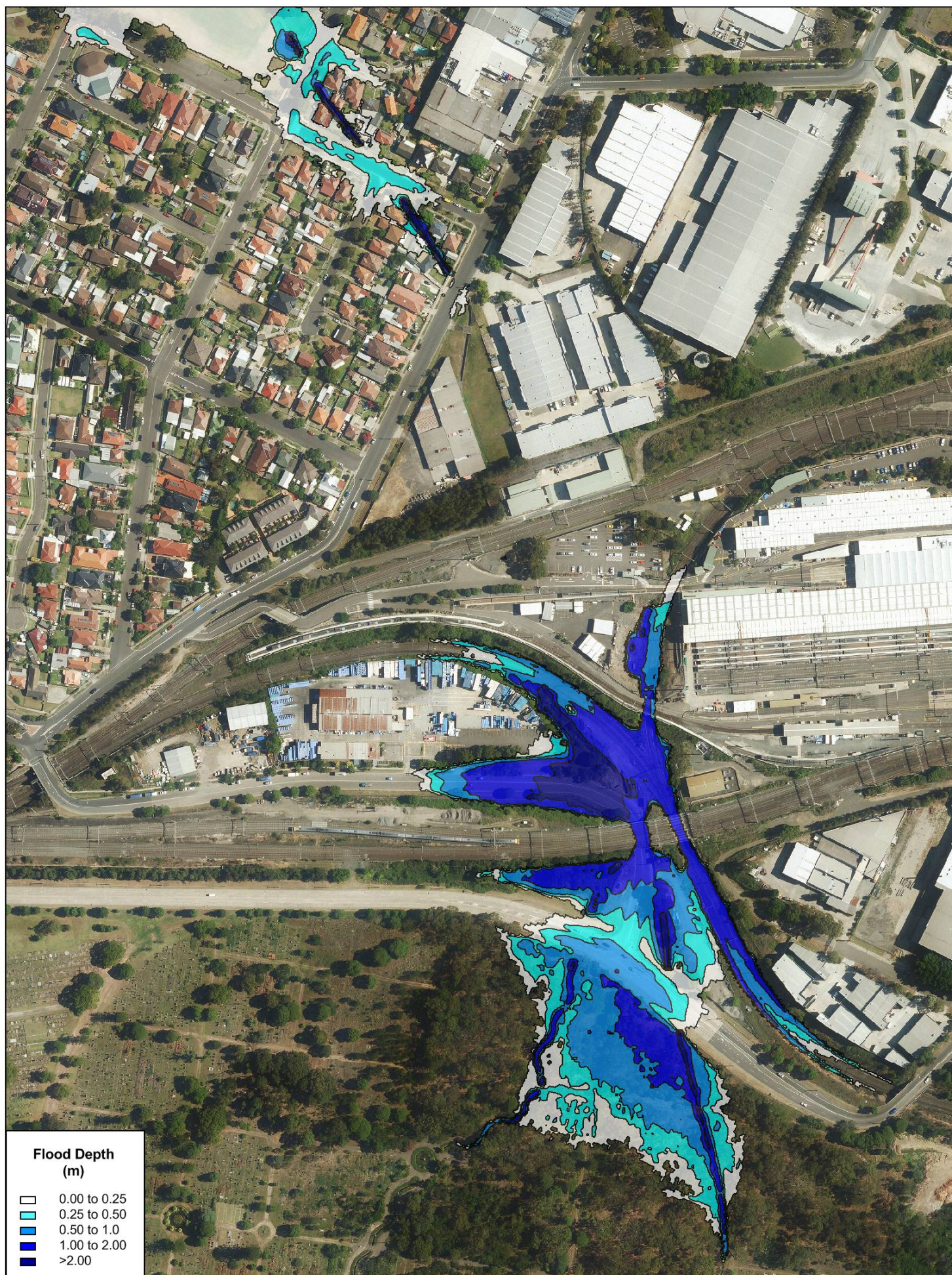
FIGURE C2 Design Scenario - 1% AEP Flood Depths
