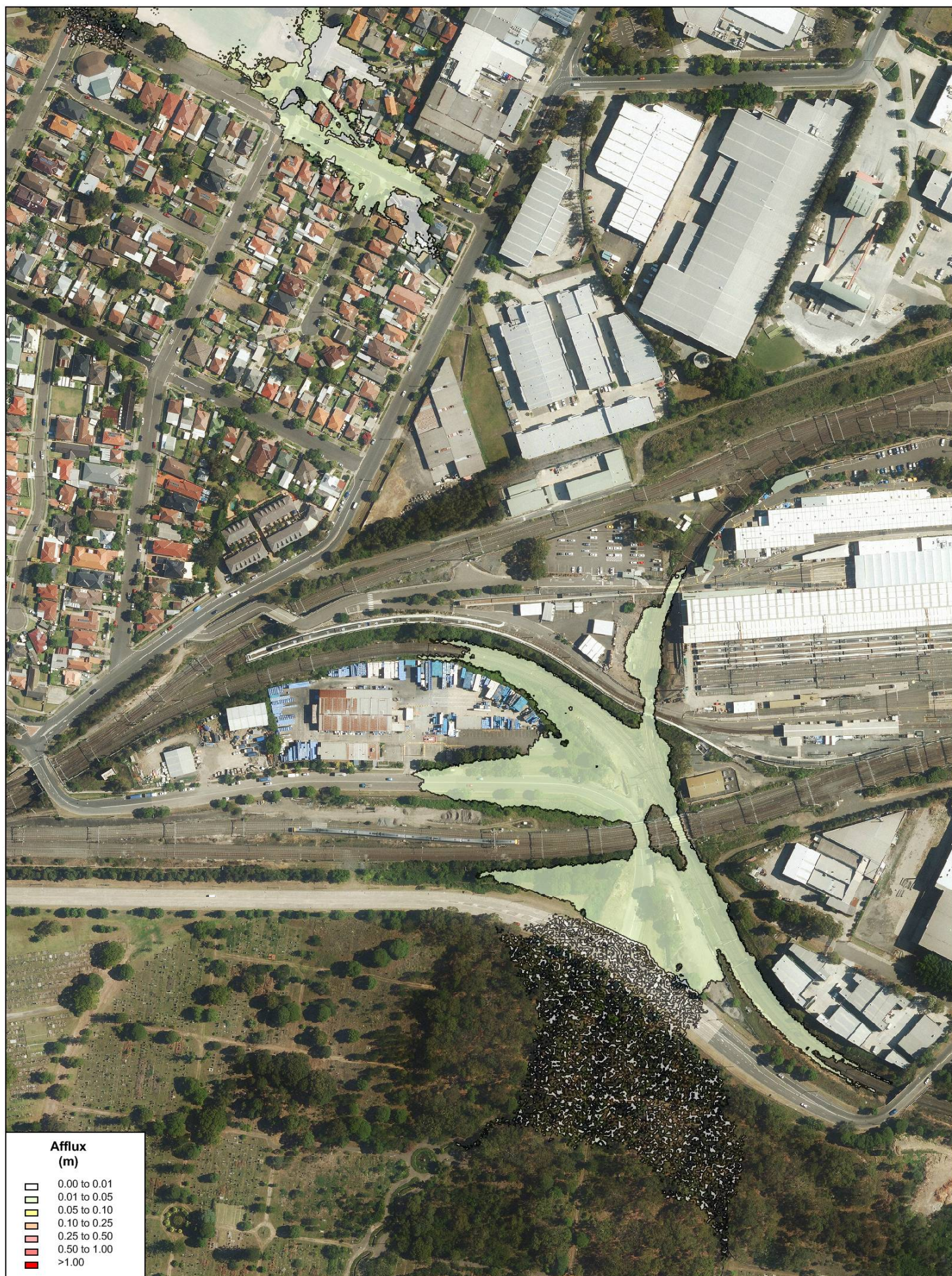
FIGURE D2 Impact Plot - Change in 1% AEP Flood Depths
