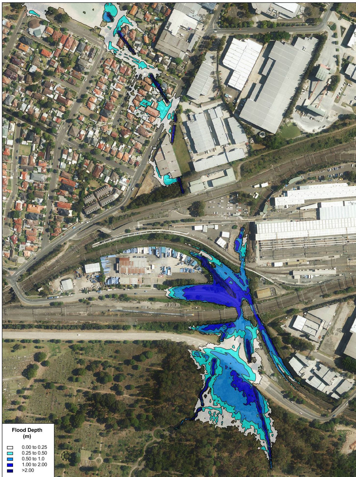
FIGURE B1 Existing Scenario - 5% AEP Flood Depths
