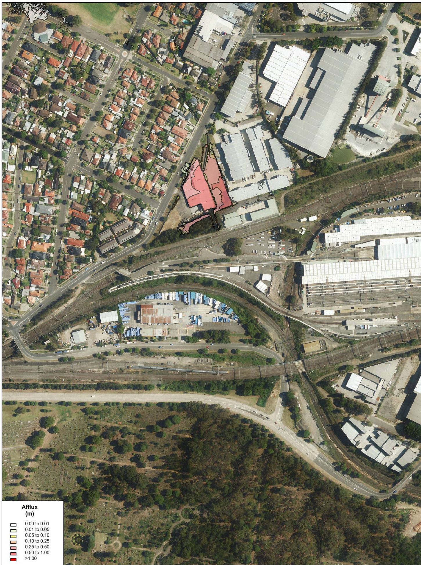
FIGURE D4 Impact Plot - Change in PMF Flood Depths
