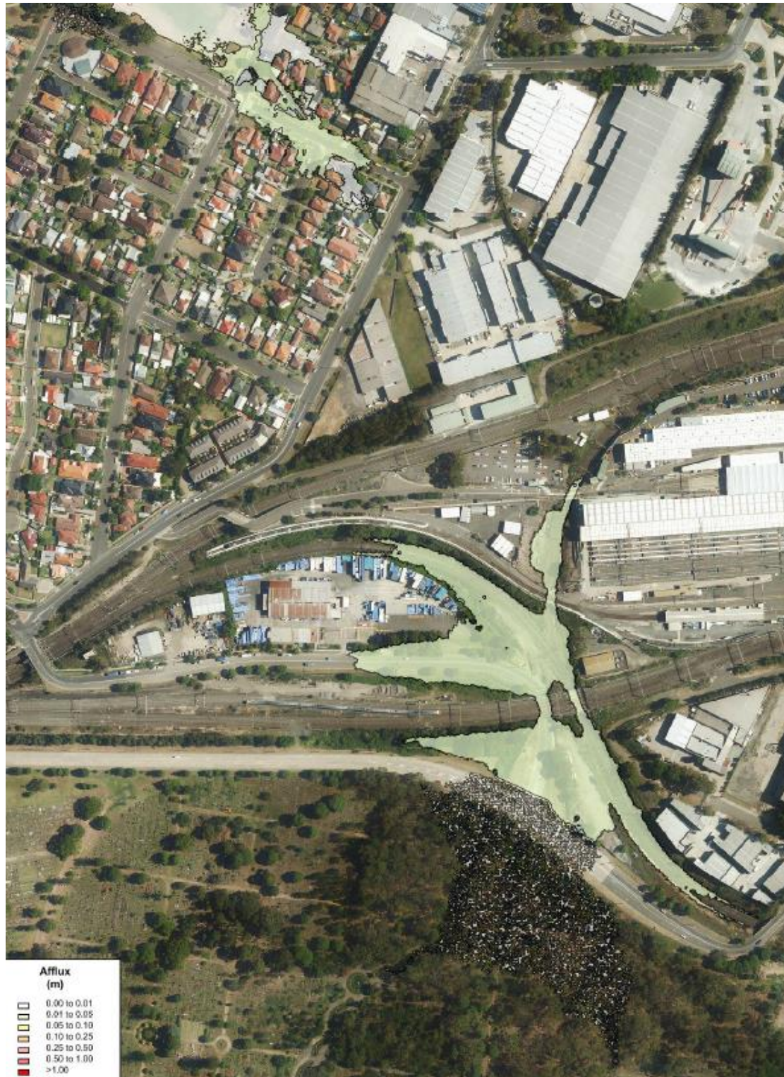
Plate 5-4 – Impact Plot: Change in 1% AEP Flood Depths
